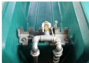
Option H : connected to water loop with 24 V-20 W-2 m heating cable. 1 MAXIFLOW float valve + 1 heating element of 24 V-180 W
