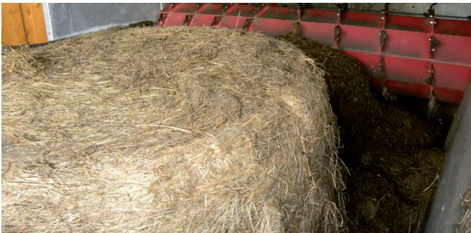
Classic FR storage bin with two milling opening rollers for small and medium-sized operations.
