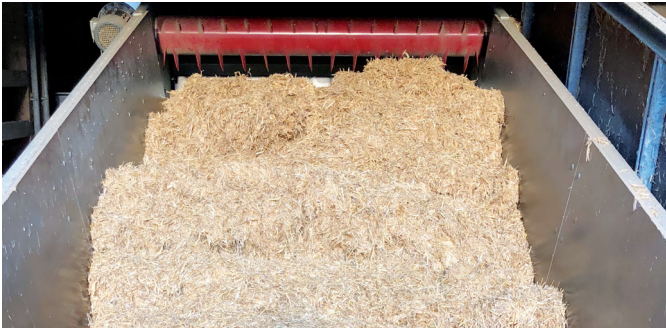
Classic 2DO storage bin with two dosing rollers and a floor scraper for small and medium farms.
