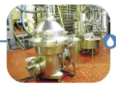
Some of the milk is separated into cream and skim milk. The skim milk is further concentrated with a reverse osmosis system, which removes some of the water in the skim milk. All the products made at the plant use combinations of milk, cream and concentrated skim milk as ingredients.
