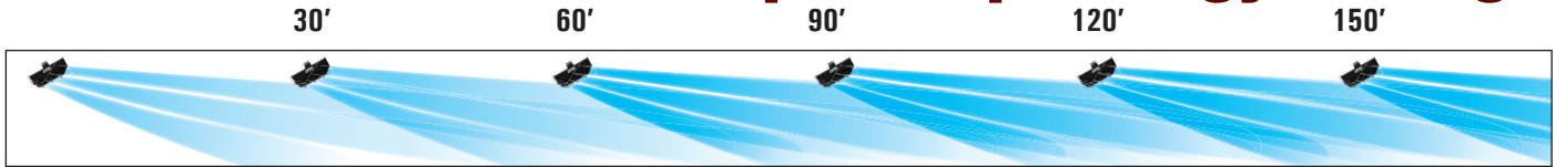
30' apart running at 50% using only 1/4 the energy will provide the near equivalent amount of air as the 60' spacing running at 100%.
